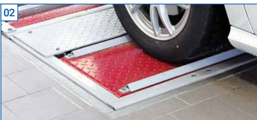
The axle damping test bench MSD 3000 is characterised by a fast and precise mechanical testing of the axle damping (Lehr's principle). The fully automatic test sequence, including the calculation of axle and vehicle weight, saves time and allows a reliable assessment of the axle damping.
