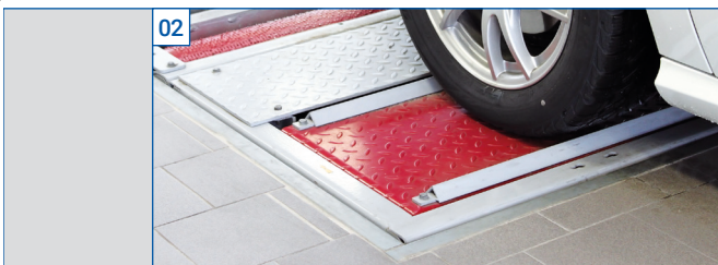
The axle damping test bench MSD 3000 is characterised by a fast and precise mechanical testing of the axle damping (Lehr's principle). The fully automatic test sequence, including the calculation of axle and vehicle weight, saves time and allows a reliable assessment of the axle damping.
