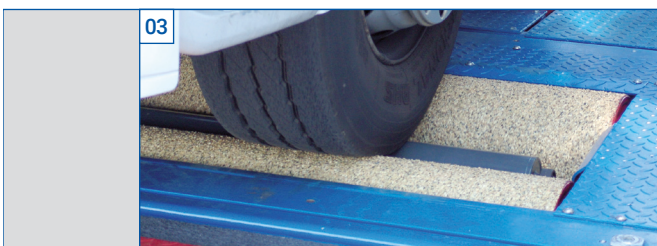
The test-lane-compatible roller brake tester MBT 7000 is designed for the brake testing of vehicles with axle loads up to 18.0 t and is ideal for vehicles diagnostics in situations of high vehicle throughput.
