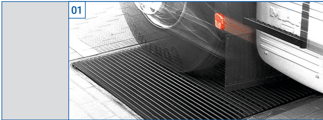
The side-slip tester MINC II EURO ensures that the axle geometry is inspected within seconds once the test vehicle passes over it (up to 15.0 t axle load) as well as a fully automatic evaluation of the deviation in m/km.
